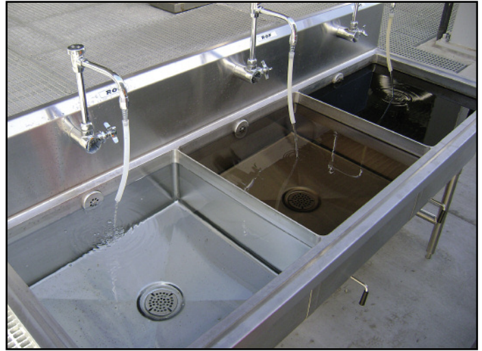
A display at the Orange County Groundwater Replenishment System (OCGRS) illustrates the effects of filtration. From right to left: unfiltered effluent; post-micro filtration effluent; post-reverse osmosis effluent.
